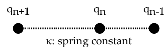
Figure 3.14: Mechanical waves in one dimension: the atoms are arranged in a linear chain and coupled with springs. q_i denotes the elongation away from equilibrium for the i -th atom.
